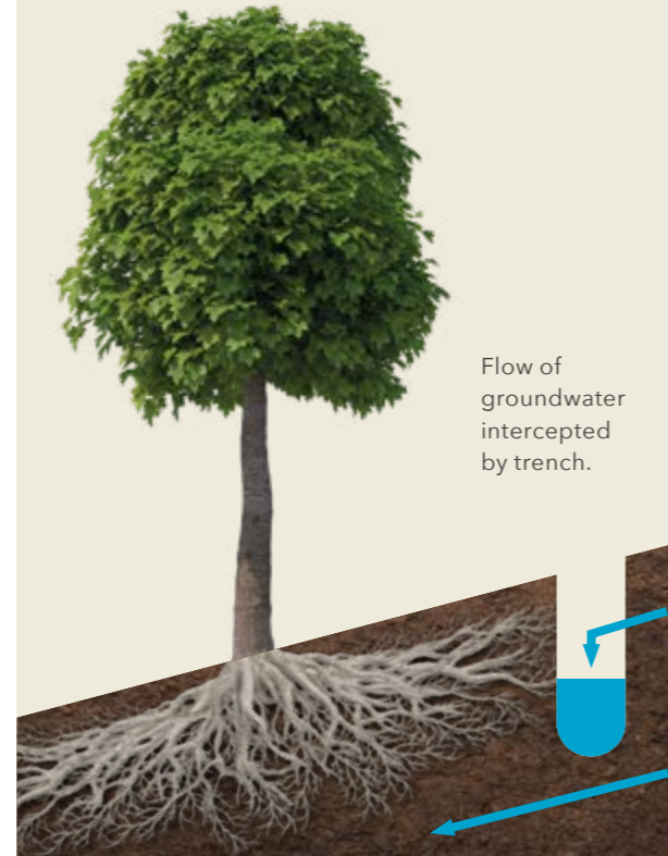
FIGURE 14: TRENCH CUT ABOVE A TREE
