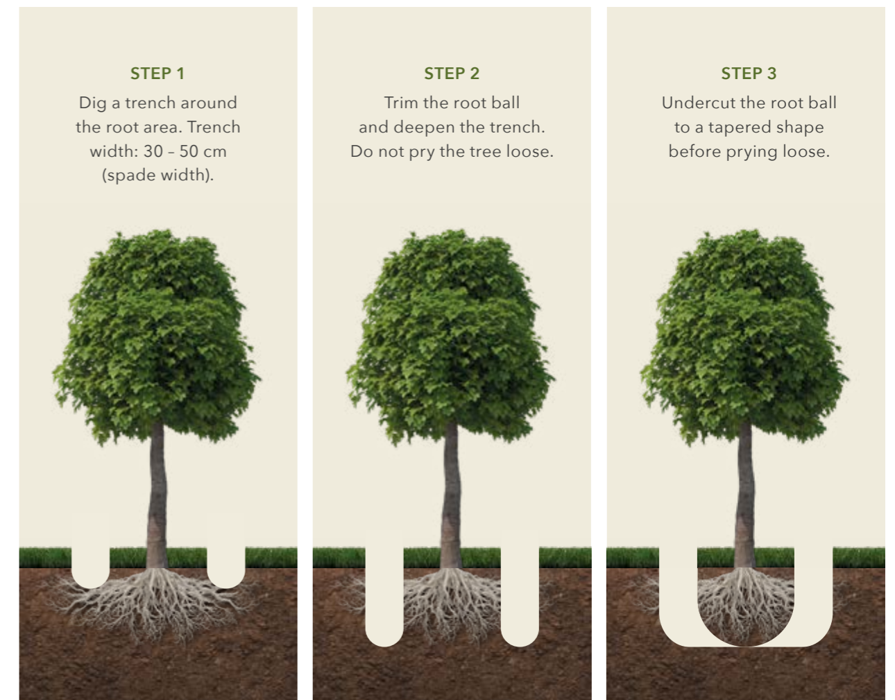
FIGURE 10: REMOVAL OF A TREE FOR TRANSPLANTING
